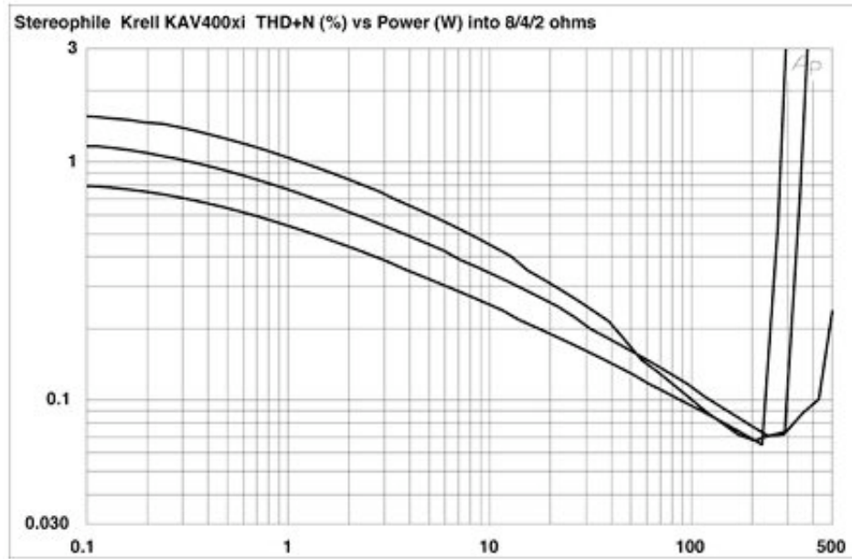
Fig.4 Krell KAV-400xi, distortion (%) vs 1kHz continuous output power into (from bottom to top at 1W): 8 ohms, 4 ohms, 2 ohms.
